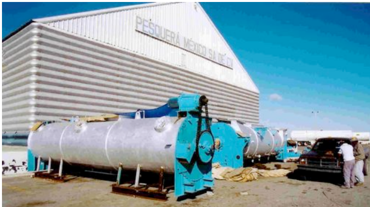
This 60 ton burner has been replaced with a 1000 ton burner at the Calmex plant. The 60 ton burner has been sold to the Moon plant, creating the capacity to burn 1060 tons per day of sardines for low quality fish meal.
